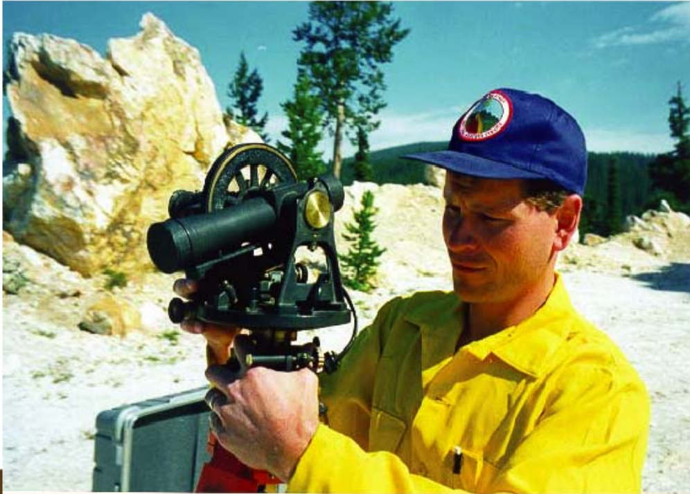
NWS Forecaster Troy Lindquist using a theodolite to track a pibal and determine the winds in the vicinity of a forest fire near Grand Junction, Colorado. The horizontal and vertical wheels display the azimuth and elevation angles of the balloon.
